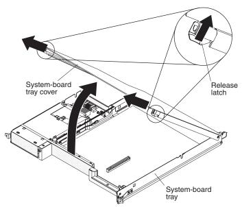
To remove the system-board tray cover, complete the following steps:
