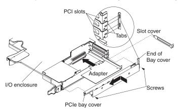
To install an outer adapter in a PCI riser card, complete the following steps:
