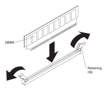
To install a DIMM, complete the following steps:
