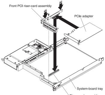
**Note:** The front PCI riser-card assembly supports installation of only half-length, full-height adapters.
