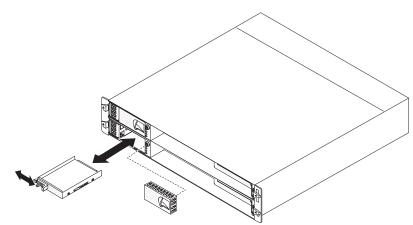
To remove a 2.5-inch simple-swap hard disk drive or solid-state drive, complete the following steps:
