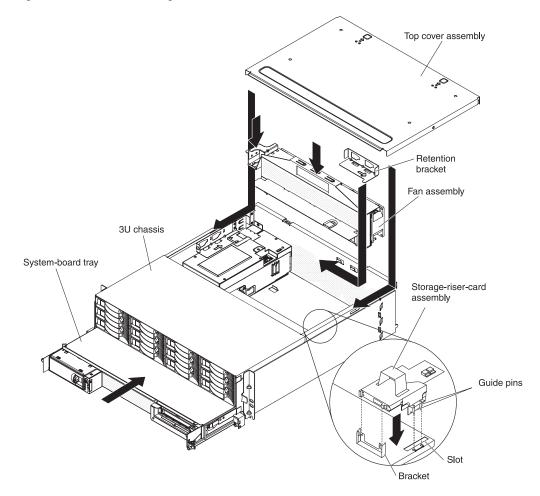
**Note:** You must remove the 3U chassis from the iDataPlex rack before you install the system-board tray (see "Removing a 3U chassis from an iDataPlex rack" on page 28).
