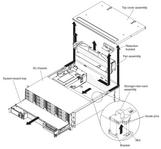
To remove a system-board tray from a 3U chassis, complete the following steps:
