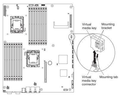
To install an IBM virtual media key, complete the following steps:
