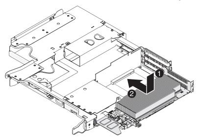
Push the card gently into the slot. Make sure that the screw holes on the card and the chassis are aligned.
