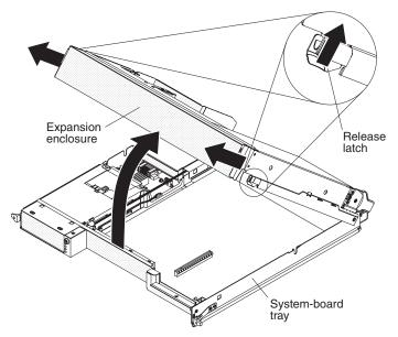
To remove an expansion enclosure, complete the following steps:
