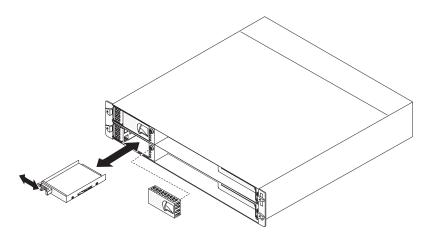
To install a 2.5-inch simple-swap hard disk drive or solid-state drive, complete the following steps:
