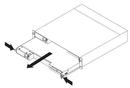
To remove a system-board tray from a 2U chassis, complete the following steps:
