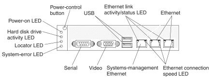
**Power-control button:** Press this button to turn the system-board tray on and off manually or to wake the system-board tray from a reduced-power state. Note that the power-control button is recessed to prevent the system-board tray from being turned on or off accidentally. There is a power-control button cover that can be removed for easier access to the power-control button.
