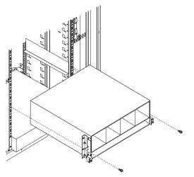
To remove a 3U chassis from an iDataPlex rack, complete the following steps:
